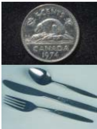
Figure 2.29 Nickel is widely used in solution with other metals to create alloys . Some coins are made of copper-nickel alloys. Stainless steel is made of iron, nickel, and other elements.
